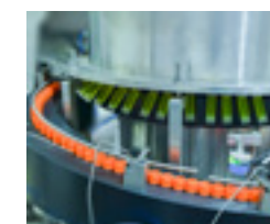
Reagent tube high-speed feeding
