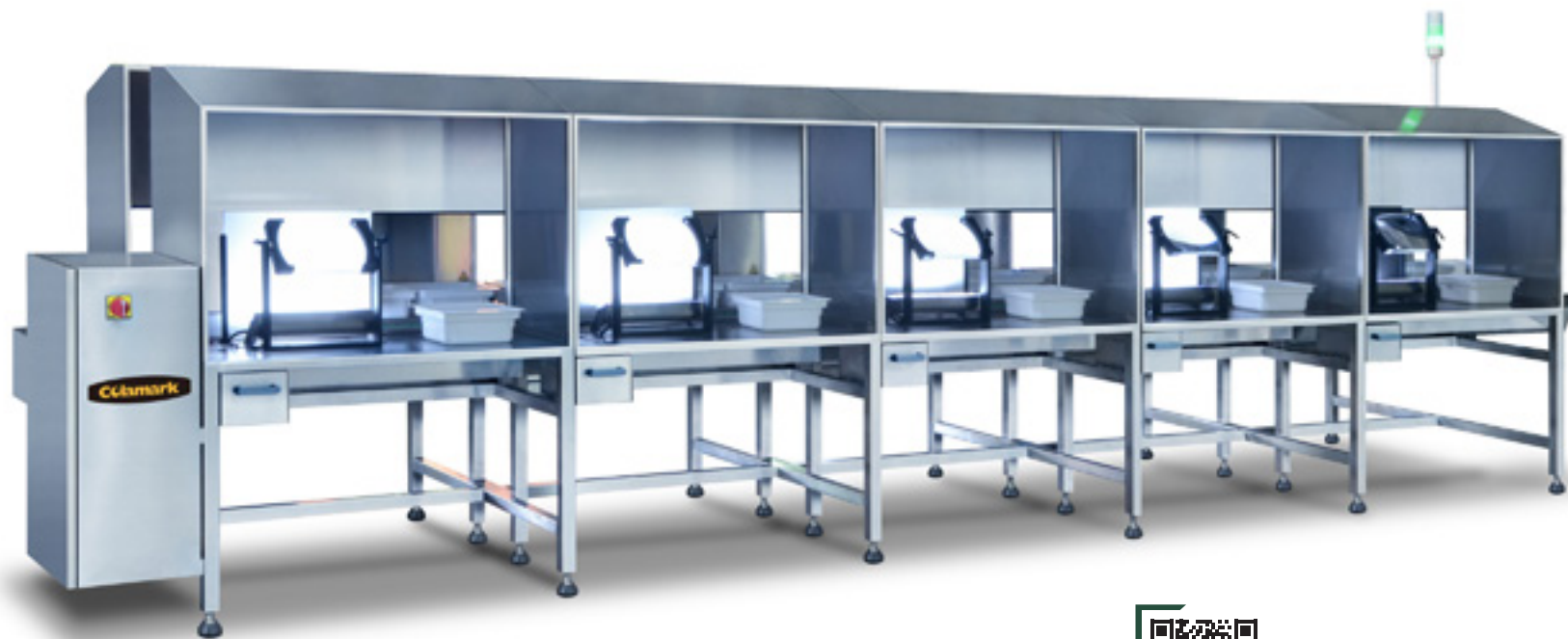
10-stations semi-automatic visual light inspection system
