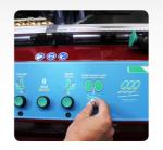
Adjustable speed control Allows quality cutting of different hardness of timbers or synthetic mouldings without changing the blades
