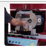
Easy maintenance Top cover can be easily opened for direct access to blades and belts
