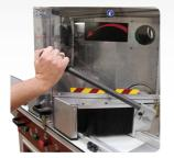
**Independent and manually** controlled cutting stroke
