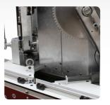
2 pneumatic horizontal clamps (foot operated)
