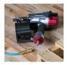
Step 1: Always Disconnect Tool from Air Supply When Not in Use
